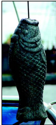
Figure 2—A 12 foot stainless steel wire with zinc on the end cast in the shape of a grouper. It is sold as a sacrificial anode to prevent galvanic corrosion. It has been repurposed to act as part of the ground system when not under way.
