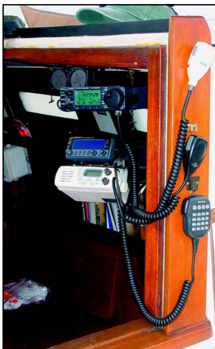
Figure 1—The control heads for three of the radios. From top to bottom: ICOM IC-706MKII used for HF, Kenwood TM-V7A for VHF/UHF and the VHF marine radio.
